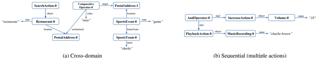
Figure 3: (a) is the AMRL for “find restaurants near the sharks game.”. (b) is the AMRL for “play charlie brown and turn the volume up to 10”. There are two actions that AMRL could handle with a sequential operator. These requests are challenging to handle using the current domain-based SLU representation.
