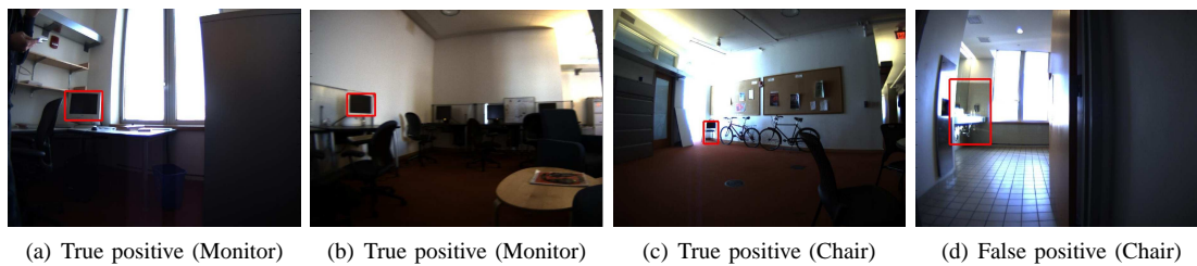
Fig. 6. Using the approach in [3], we classify a number of categories in the an office building on MIT. Above are some of the images classified correctly and one instance of a false positive. In (a/b) are the two locations where a monitor was detected in the environment. In (c) is a true positive of a chair while in (d) is a false positive of a chair.
